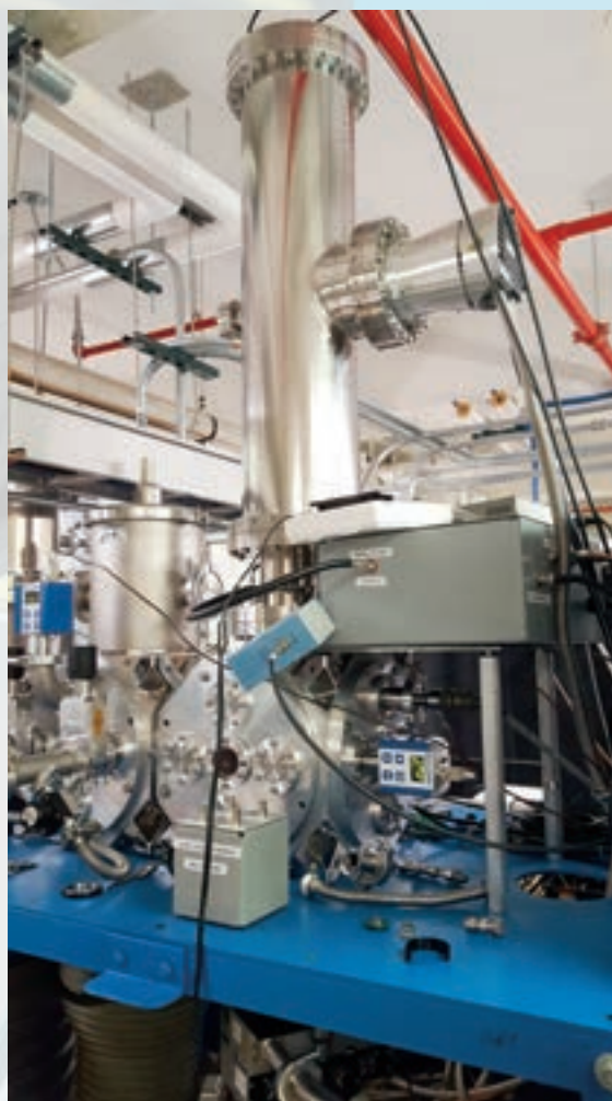
Helium droplet molecular beam machine and mass spectrometer in Prof. Gary Doublerly's lab
